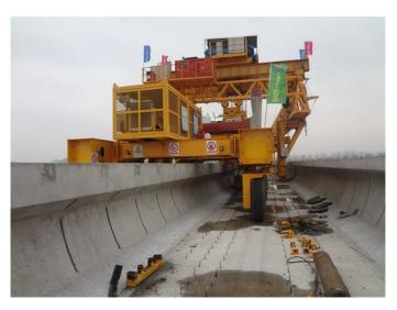
Wheels are powered by hydraulic motors and steering is by means of hydraulic cylinder. Driver Cabin is provided and wireless control system is part of the supply for convenience of contractor. Safety features are always main consideration of Huada Heavy Industry equipment. Limit switch, emergency break switch at varies location, sensors, auto alignment system etc. are part of the safety controlling device that installed in the transporter.
