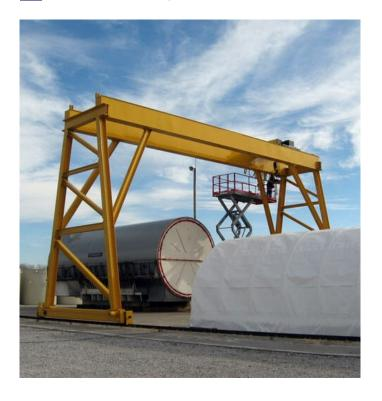
Gantry Crane is widely used outdoor on the big work yard to lift material. There is no need to install the steel stand column, therefore, Gantry Crane will not occupy too much ground space.
