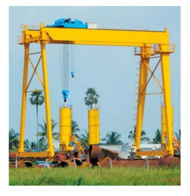
Double girder Gantry Crane is mainly consisting of the gantry structure, lifting trolley and cross traveling mechanism, long traveling mechanism, cabin and electrical control system. The trolley can move horizontally on a pair of rails on the main girder. The girder can be box or trussed type in according to working environment situation.
