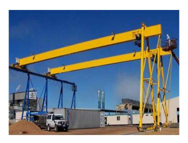
Semi Gantry Crane compared with electric single-girder crane, save investment and space, compared with electric hoist gantry crane, save the production space, therefore when selecting ordinary electric single-girder crane or electric hoist gantry crane is not very ideal, semi gantry crane is a better solution.
